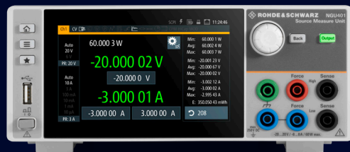
R&S®NGU401 four-quadrant source measure unit.
