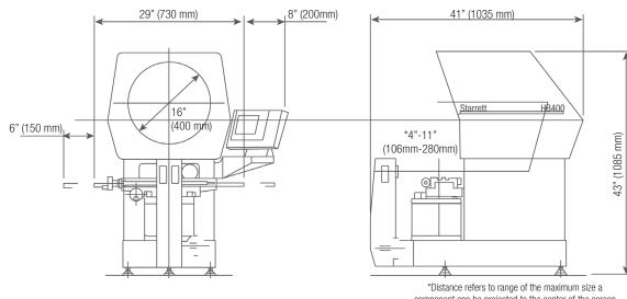
\*Distance refers to range of the maximum size a component can be projected to the center of the screen before colliding with the lens. (100X-10X)
